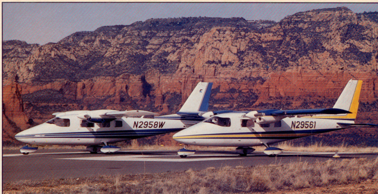
Turbo P-68C, left, has different paint and engine cowlings, but its real difference from the Victor is evident in a high/hot takeoff.
